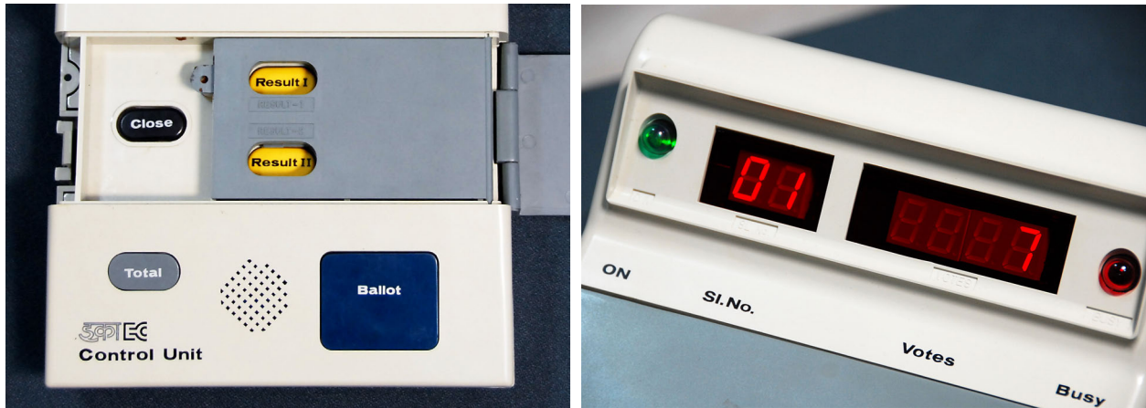
Figure 2: Counting Votes — The EVM records votes in its internal memory. At a public counting session, workers remove a seal on the control unit and press the RESULT I button ( left ) to reveal the results. The machine sequentially outputs the number of votes received by each candidate using a bank of 7-segment LEDs ( right ). Here, candidate number 01 has received 7 votes.
