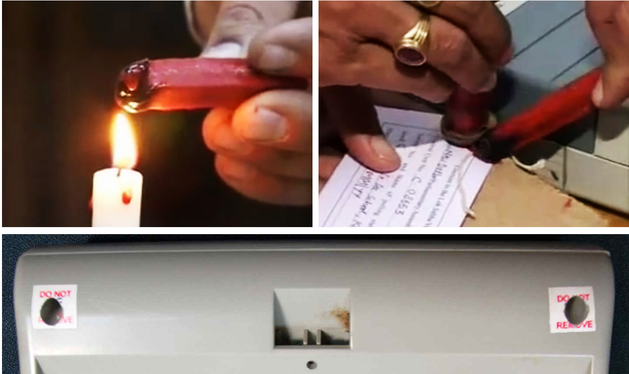
Figure 9: Tamper-Evident Seals — Frames from an official training video [45] show how poll workers seal the control unit doors using red wax and string ( top ). The paper tags are signed by candidates’ representatives, but these signatures are not routinely verified. Seals placed over screw holes on the underside of the control unit ( bottom ) consist of printed paper stickers. All these low-tech seals can be easily faked and provide extremely weak protection.
