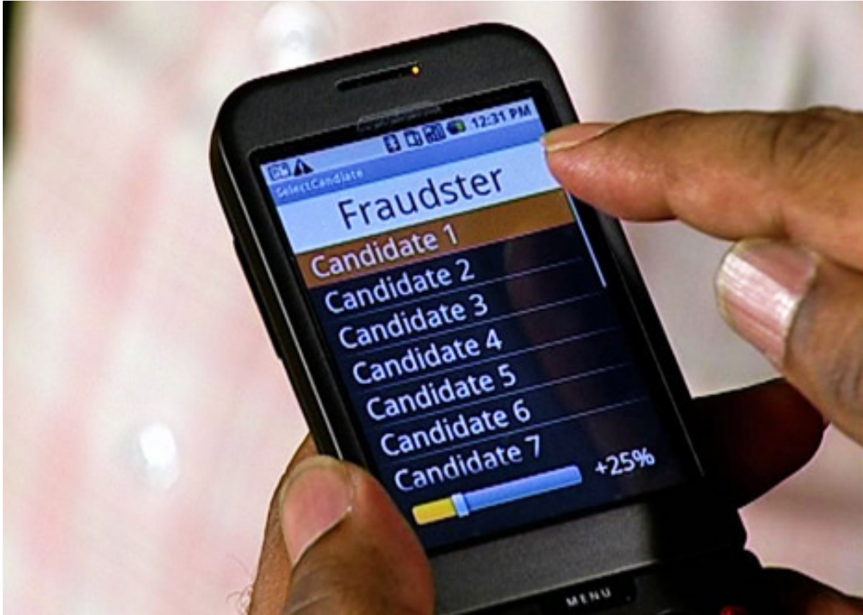
Figure 6: Wireless Signaling — An application running on an Android mobile phone uses Bluetooth to tell our dishonest display which candidate should receive stolen votes. Attacks using other forms of radio communication are also possible.
